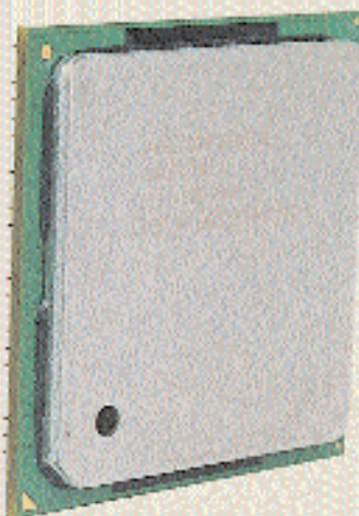
The Pentium 4's Thermal Heat Spreader protects and dissipates heat from its core
